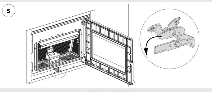
Close the insert and block the latch.
