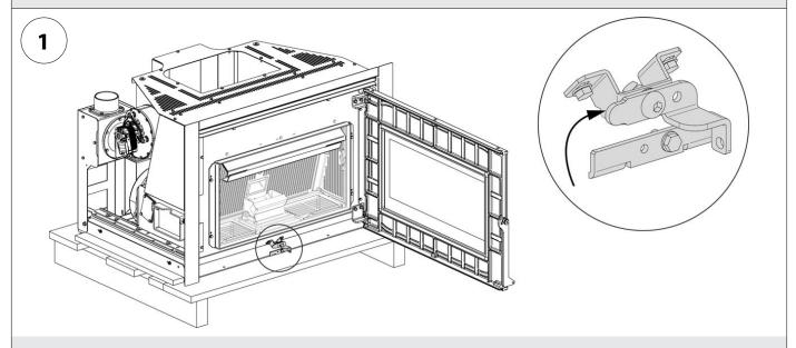
Open the door and release the latch using the poker supplied.
