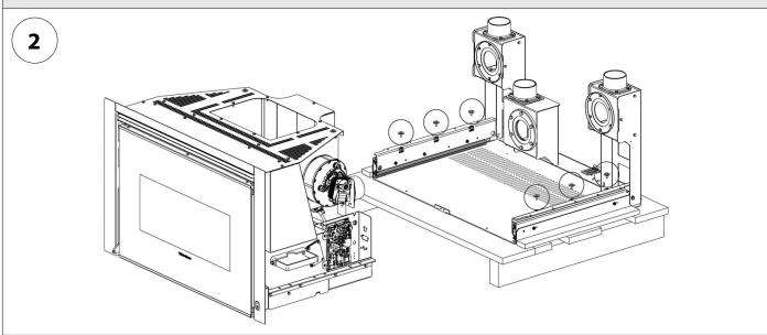
Remove the 6 screws and remove the flue pipe from the base.
