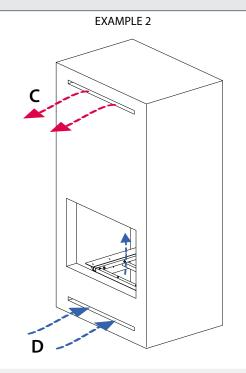
**C**: Air convection outlet. Minimum section 240cm<sup>2</sup>. **D**: air inlet from room. Minimum section 240cm<sup>2</sup>.
